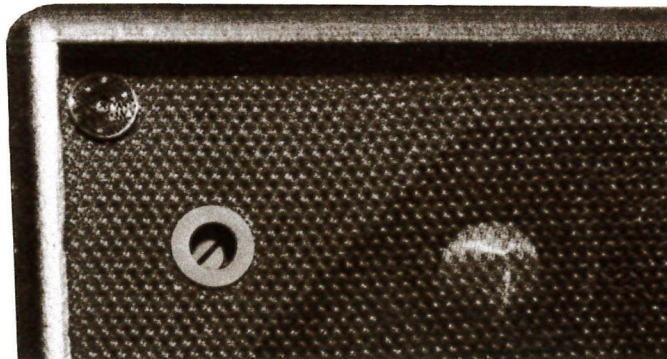
Figure 5. High frequency attenuation control.
